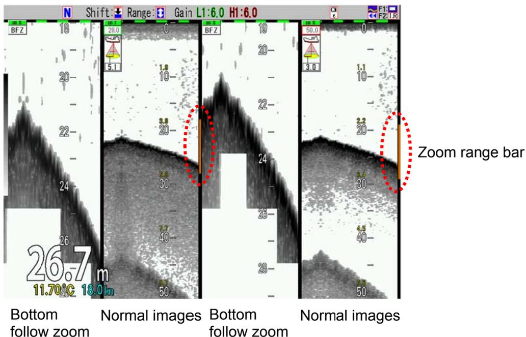
In a specified zoom range, the sea bottom is displayed by automatic shift to be displayed within a range between 30 % and 90 % from the top of images
