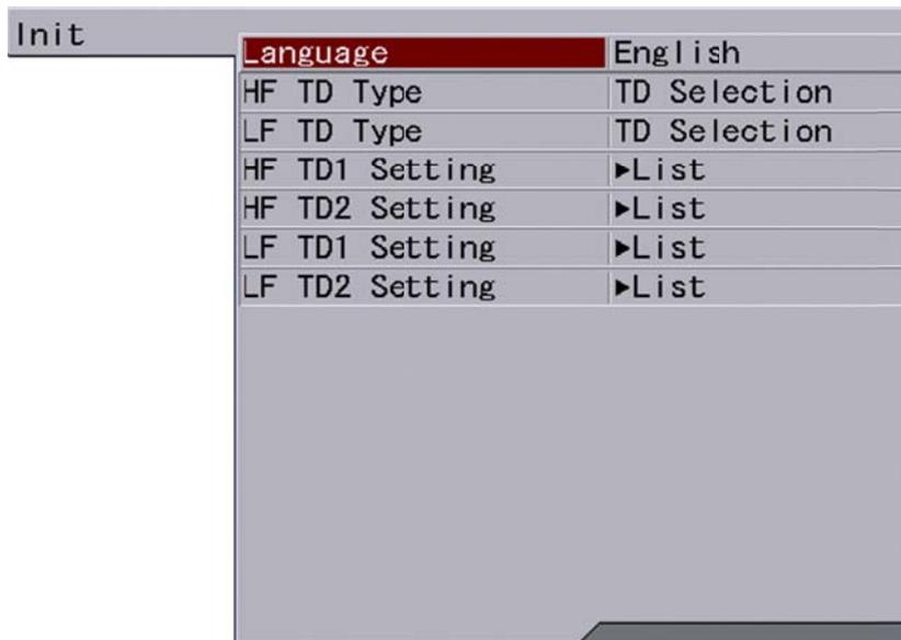
Set [TD type]. (Refer to the Installation Manual “2.1 Setup of transducer” of “Chapter 2 Adjustment”)
