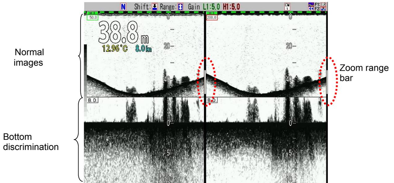
Sea bottom is fixed at 30% bottom of the screen, and the image of bottom is displayed in the specified zoom range.
