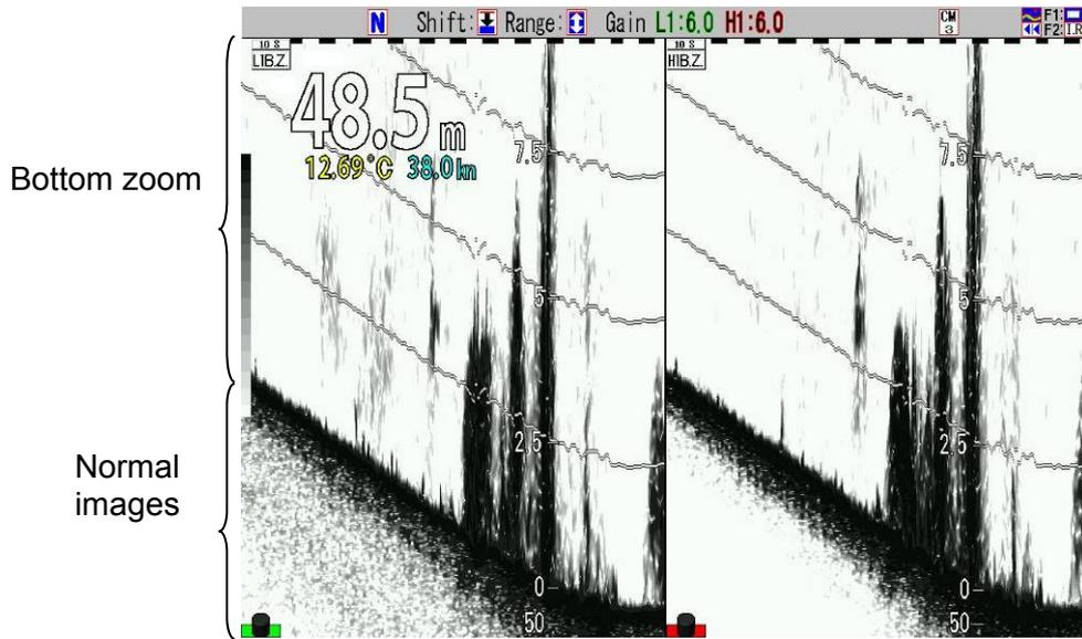
Mixed images above bottom in a specified zoom range are displayed onto the normal image.
