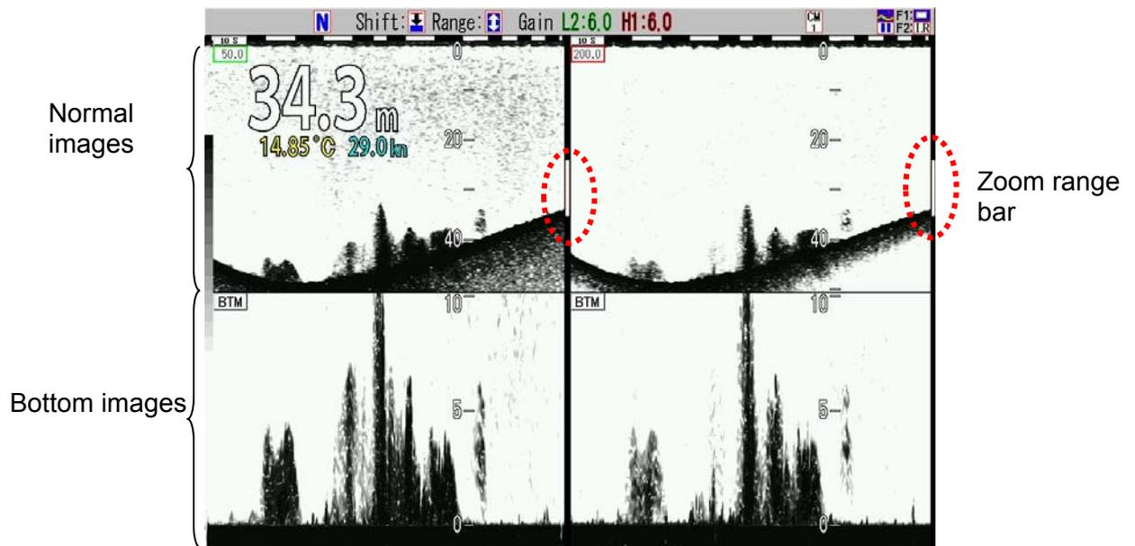
Sea bottom is fixed at 10% bottom of the screen, and the image above is displayed in the specified zoom range. As the image on sea bottom is magnified, this is an effective zooming mode to identify fish schools, etc. near the bottom.
