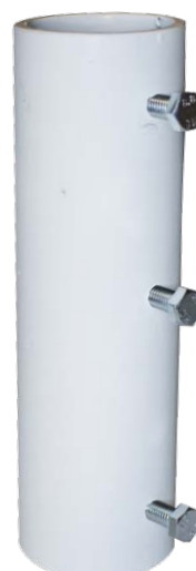
Pipe adaptor Steel tube, open ends, 50mm inner diameter/60mm outer diameter, 3pcs M10 lock screws, weigh 1,4kg, length 20cm (to fit 64mm U-bolt to smaller than 50mm diameter vertical pipe)
