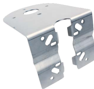
Antenna mount adaptor 3 140mm proTAC flange to wall or 50-75mm horizontal/vertical pipe A4 stainless steel
