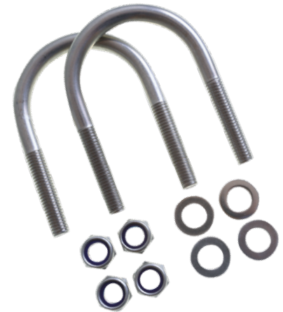
A2 stainless steel U-bolt kit for ACCANT1003/1006 (2 pcs M12/76mm U-bolts, 4 pcs washers and bolts)to fit 64mm pipe
