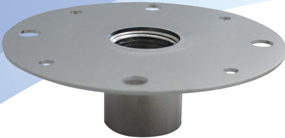
Antenna Mount adaptor 1 140mm proTAC flange to BSP1"-11TPI pipe thread (R1 inner thread) A4 stainless steel
